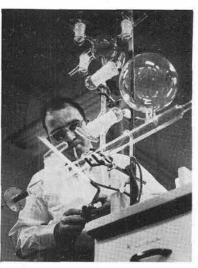
RON SNIDOW, Glass Shop supervisor, applies final touches to a glass vacuum manifold fabricated for Division 4411. Typical of the laboratory apparatus created by the Glass Shop, this piece demonstrates the skill of the glassblower.
